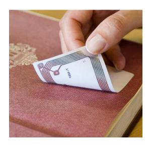
KSmart-RFID Tags are specially designed for library application. These ultra-thin, flexible HF ISO tags with an electronic chip are applied on Books / CDs/DVDs and can be read without contact and line of sight. RFID Tags have inbuilt EAS / AFI function to ensure detection against thefts and are designed to last lifetime of the item they identify. RFID Tags have lockable section for item identification, re-writable section for library use and security function.
